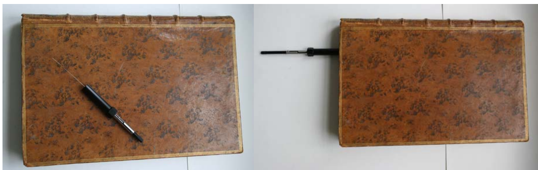
Figure 14. (Left) SPME fibre ; (Right) the SPME fibre inserted in a book to sample the VOCs emitted. (Photo credit: A-L Dupont, CRC-MNHN)
