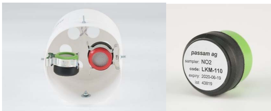
Figure 15. Passam Ag diffusion samplers
