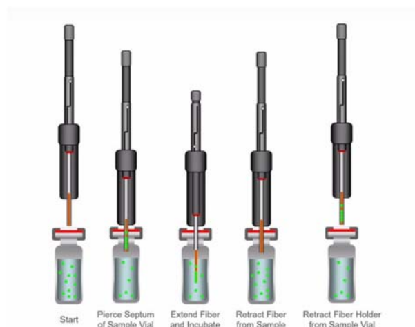
Figure 13. SPME fibre in headspace sampling mode in a small vial ( Agilent )
