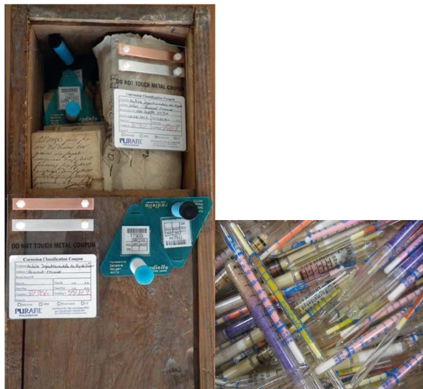
Figure 16. (Left) Exposure of Purafil coupons and Radiello® tubes in an archival box from Puy-de-Dôme French Provincial Archives (Figure 4 in Dubus et al. 2015 119 ). (Right). Used Dräger and Gastec used detection tubes (Photograph credit: J. Tétreault, CCI)
