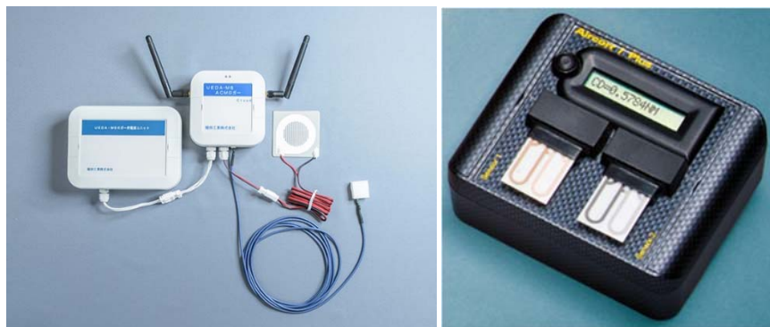
Figure 17. (Left) Radio Wave Type Monitoring Unit for a corrosion-based sensor; (Right) AirCorr corrosion monitoring system equipped with Ag-50 nm and Cu-50 nm sensors (Fig 1 in Kouril et al 2014 120 )
